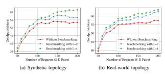
Fig. 10. Goodput v.s. number of paths in the routing table.
